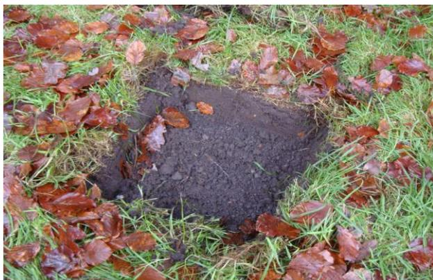
**Step 1** With a spade remove a small patch of the top vegetation layer to expose soil layer before doing the test.
