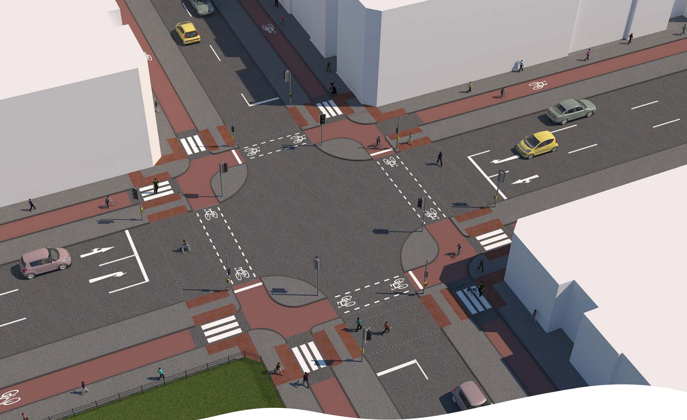
Figure 5.12: Protected signal-controlled junction layout with Zebra crossing of cycle track (3D)
