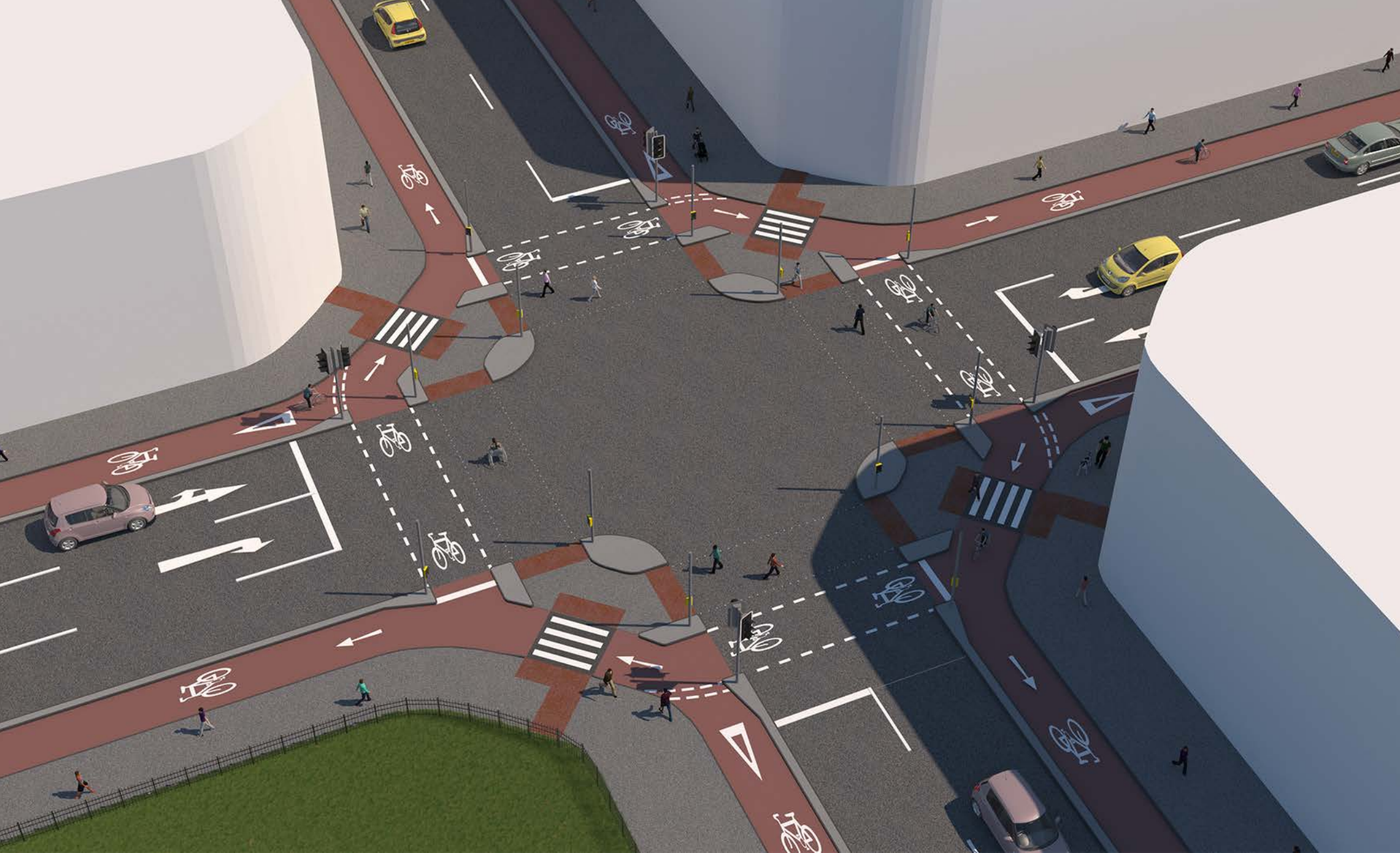
Figure 5.14: CYCLOPS protected signal-controlled junction layout with Zebra crossing of cycle track (3D)
