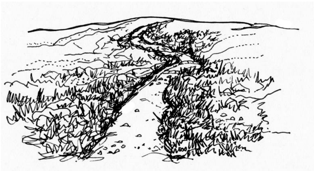
After - alignment defined, use contained, slope stabilised, vegetation restored.
