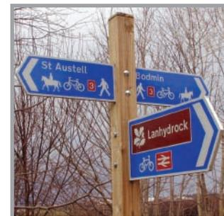
Figure 15: Example of a junction sign, in a rural area, National Route 3. Note: it is always best to include distances as well as destinations
